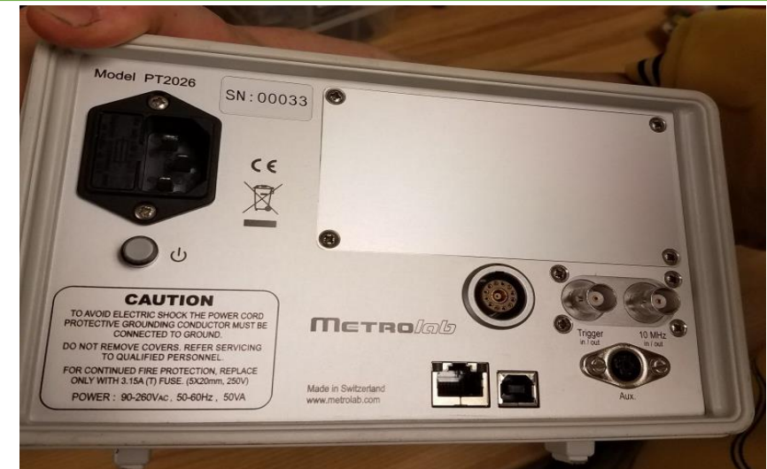
Metro-Lab PT2026 NMR unit
