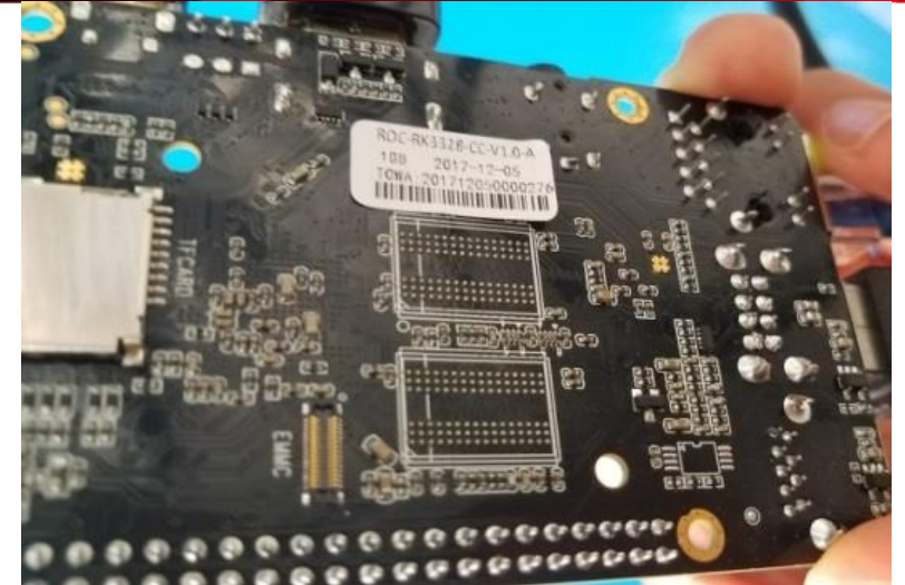
ROC-RK3328-CC SBC card implemented on Hall C control systems
